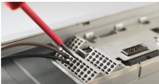
Spring loaded cage clamps are specially designed for the AutomationDrive series. Press, place, release and you have a reliable and stable connection that never needs service attention.
