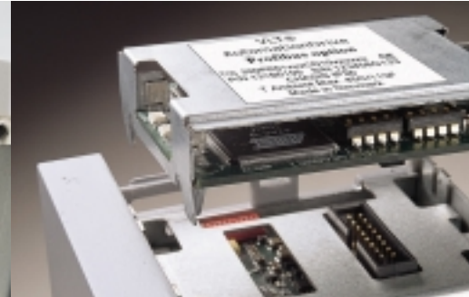
The bus option ready to plug in underneath the front panel. It can be turned upside down if you prefer the cable to enter from the top.
