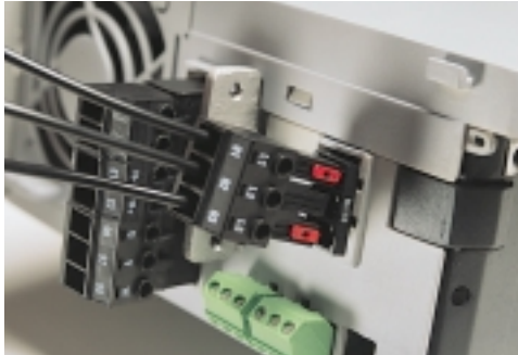
Plug-and-play is the general approach in the VLT® AutomationDrive. Even power supply, sensor cables and looping connections are gathered in plugs.
